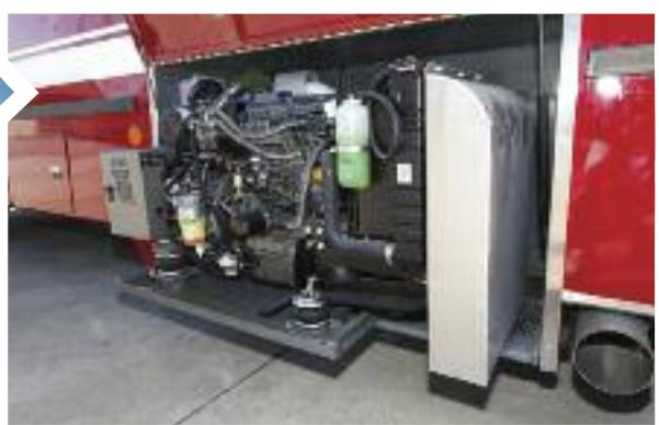
20KW diesel generator slides out for easy maintenance
